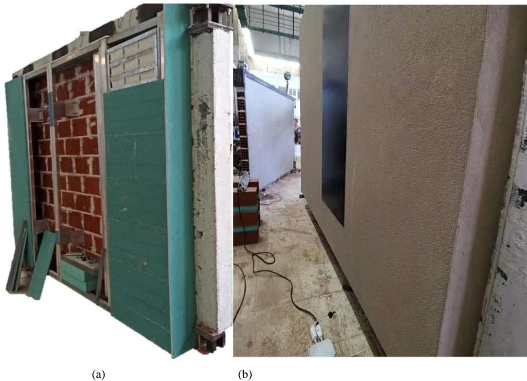
Figure 2. Presentation of under evaluation ventilated facade, (a) construction phase and (b) final configuration, PV mounted, radiation lamp and automation installed.
