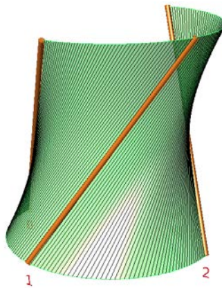
Figure 12. Regulus through three straight lines (one-sheet hyperboloid).
