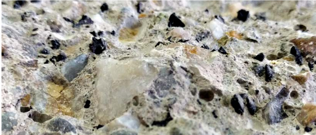
Figure 3. Specimen fracture surface of SCC mixture made with CR as partial replacement of fine aggregate and 100% coarse RCA
