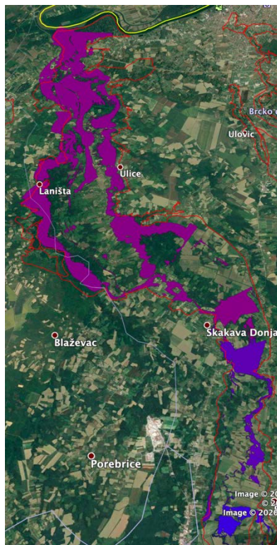
Figure 17. Calculated flood zones (areas filled with various colors) and APSFR limits (red lines) for Tinja River
