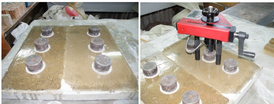
Figure 2. Surface with, and without quartz filler (left) and the apparatus used (right)
