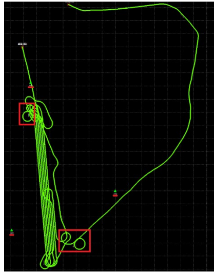
Figure 3. Flight trajectory display during recording with marks for initial turns and permanent stations [17]
