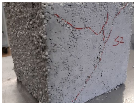
Figure 8. Compression test - failure patterns
