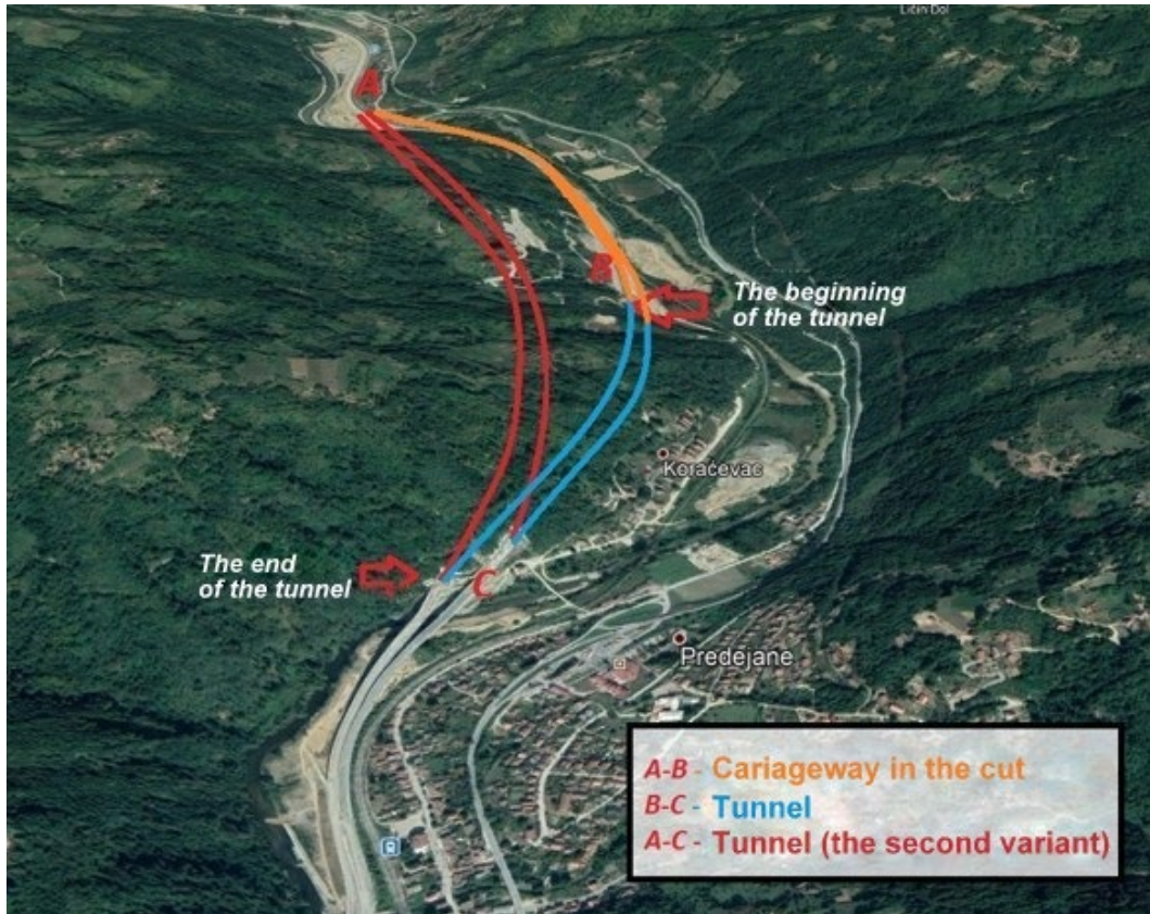
Figure 5. Tunnel tube extension
