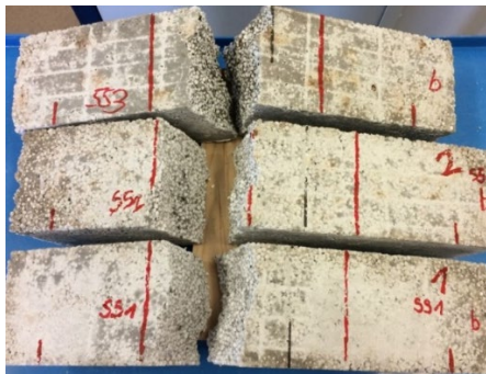
a) Typical failure mode
