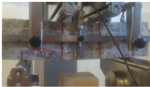
c) Crack initiation
