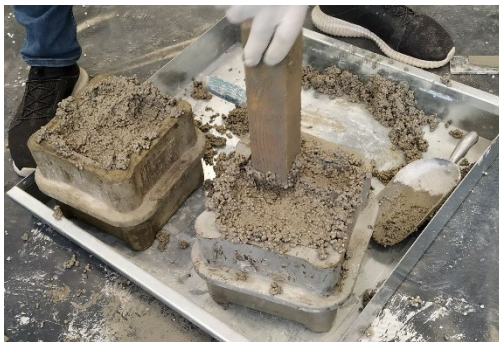
Figure 3. Casting of fresh concrete
