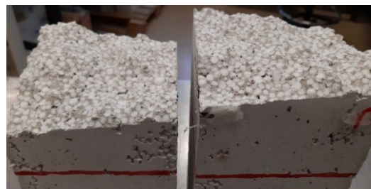
b) Failure surface
