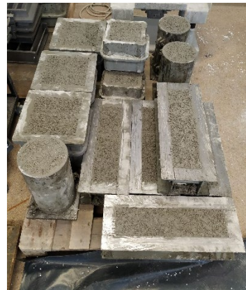
Figure 4. EPS3 concrete specimens
