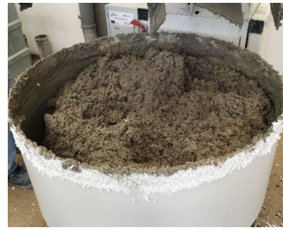
Figure 2. Fresh concrete mixture
