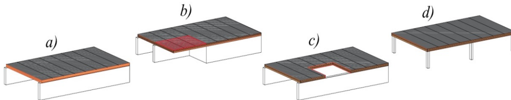
Figure 1. Different support systems of CLT floors: (a) standard beam-like structure (b) balcony; (c) rectangular opening; (d) point supports
