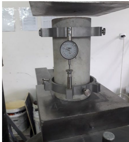
Figure 7. Measuring of modulus of elasticity
