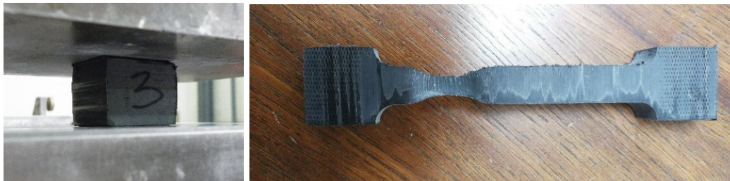
Figure 2. The appearance of the samples after failure in cases of testing compressive strength (left) and tensile strength (right)
