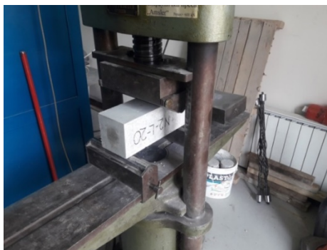
Figure 5. Three point bending test
