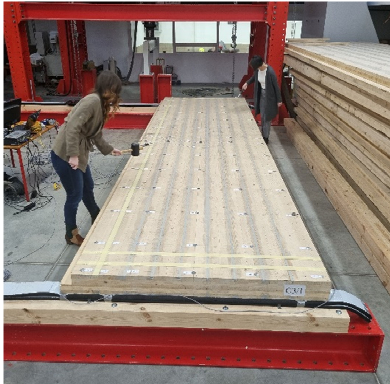
Figure 15. Modal testing of hybrid FRP-CLT panel
