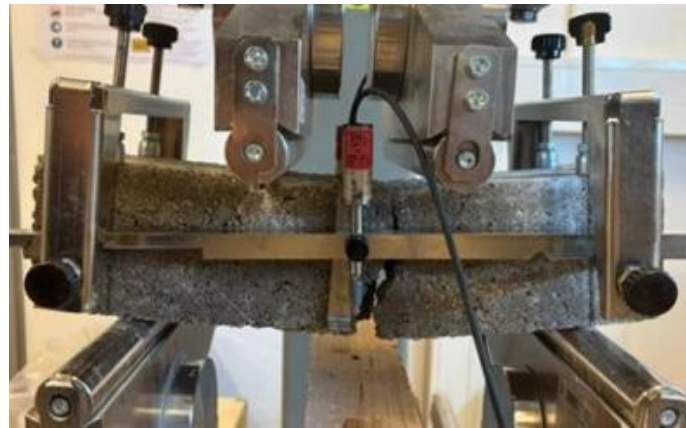
Figure 9. Flexural tensile strength testing using the displacement-controlled method
