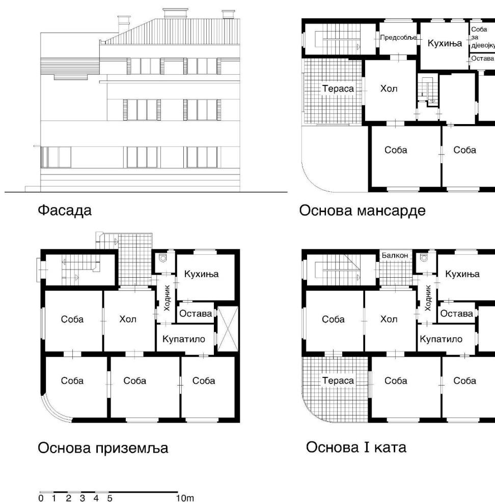
Figure 4. Floor plans and street elevation of the Draga Milošević House (Drawing by S. Cvijić)
