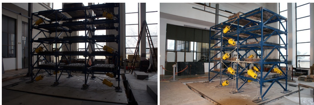
Figure 5. Tested models with PDDs on the shake table (photography by author).
