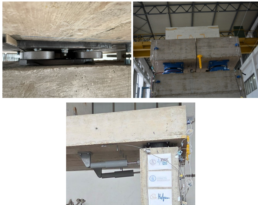
Figure 2. Somma device (left), EPS systems (right), Viscous dampers and Rubber Bearings (photography by author).
