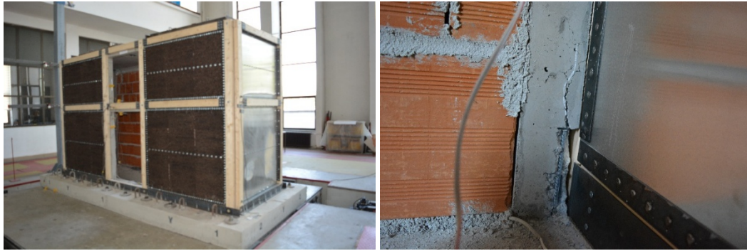
Figure 4. Model strengthened with exoskeleton (left), damages from shake table tests(right) (photography by author).
