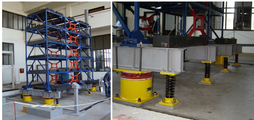
Figure 10. Model on shake table with GERB-BSC system (photography by author).
