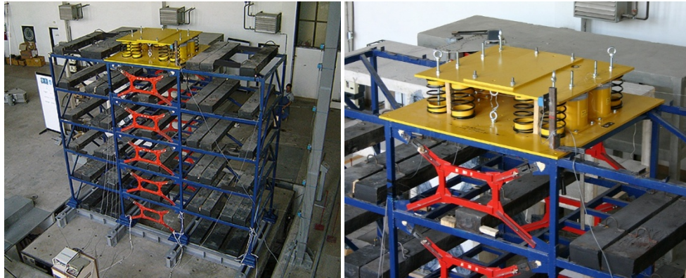
Figure 7. Tested structure with TMD (photography by author).
