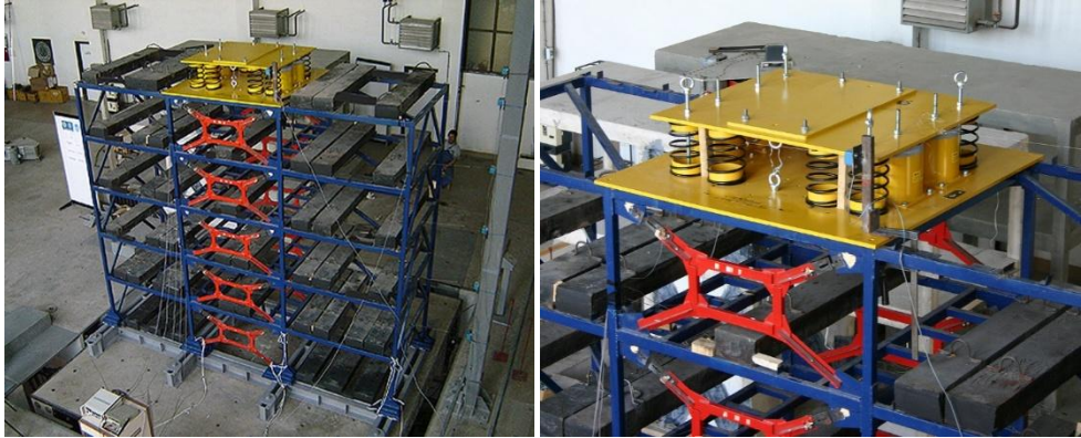
Figure 7. Tested structure with TMD (photography by author).
