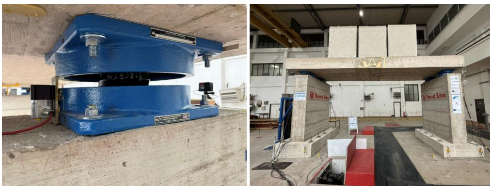
Figure 1. EPS systems implemented on the bridge model and tested on shake table (photography by author).
