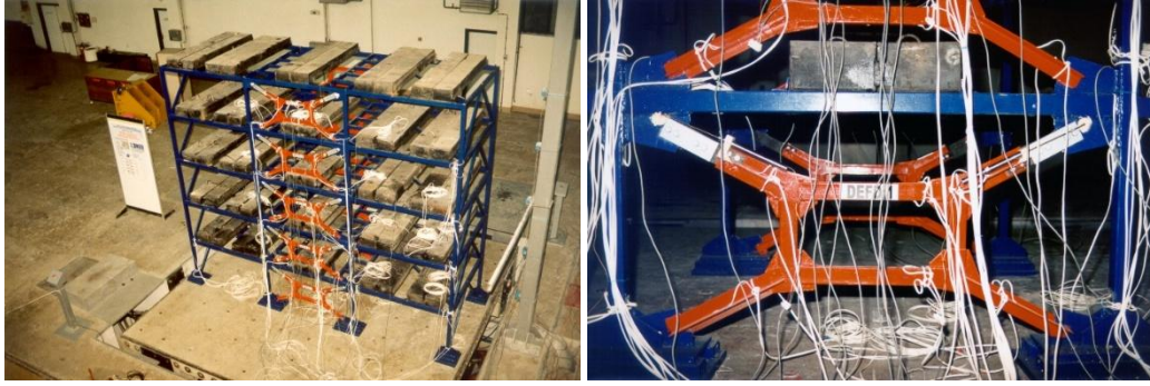
Figure 13. DEFD system on the shake table (photography by author).
