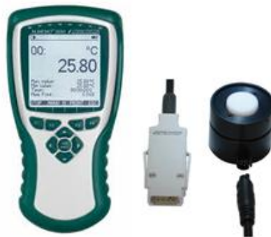
Figure 2. Almemo Ahlborn 2690-8 (left), luxmeter (right) (photography by author).
