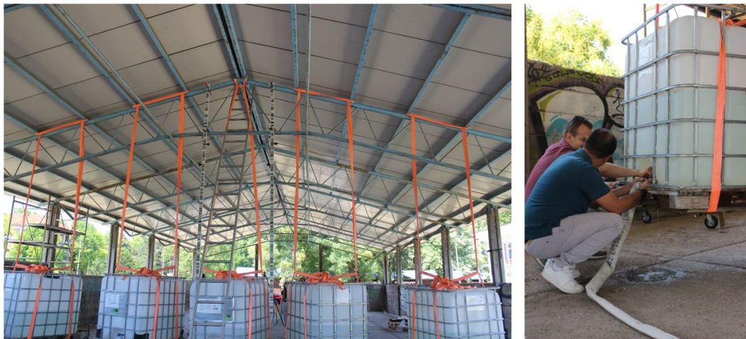
Figure 13. Proof load testing of the 'Campus garage': load application on the steel truss (left) and container unloading (right) (photography by author).
