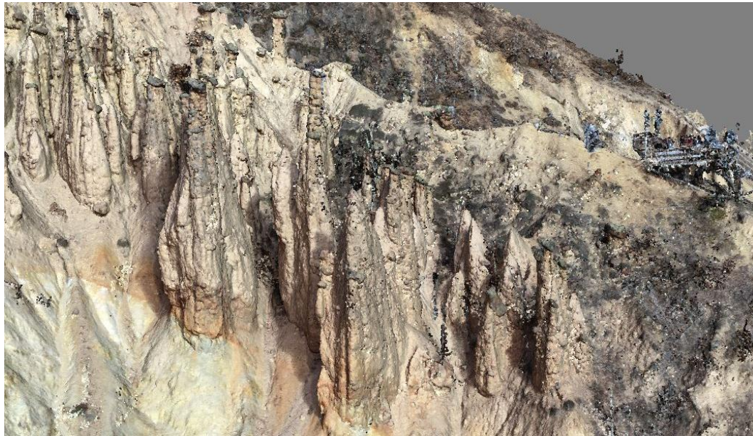
Figure 4. High-density point cloud representing the earth pyramids with fine details
