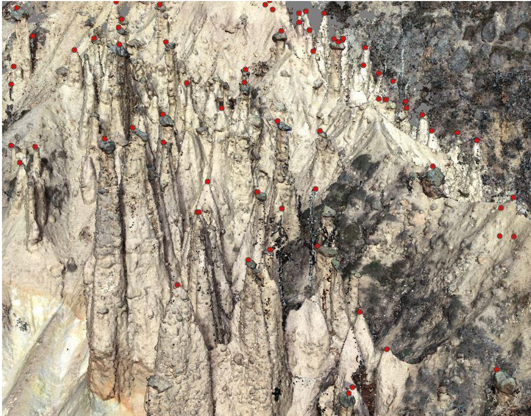
Figure 6. Detected apex points of the earth pyramids visualized in the 3D point cloud (created by author).
