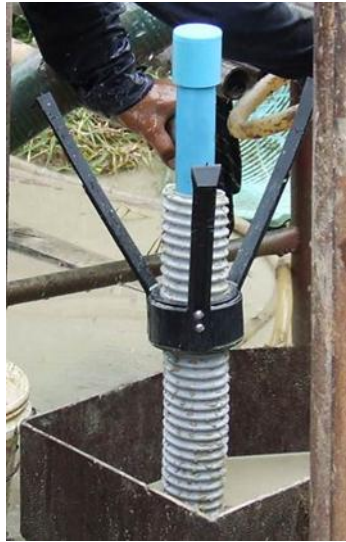
Figure 2. Corrugated pipe, lead column and "spider" spacer [21].
