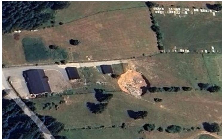
Figure 1. Crater on the surface of the terrain as a result of the collapse in tunnel (photography by author).
