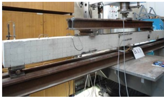
Figure 1. Test setup of the continuous beam (photograph by author).
