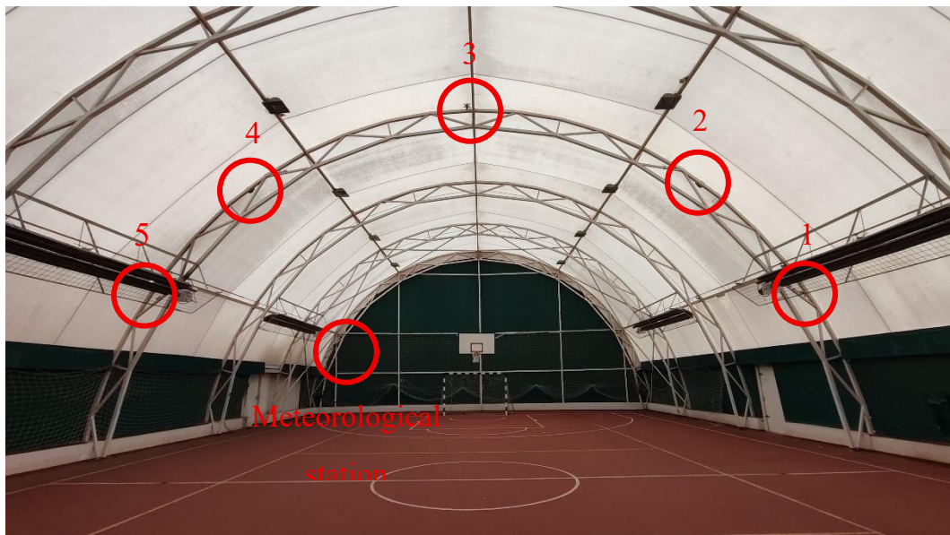
Figure 5. Set-up of the measuring devices inside the facility (source: photograph by authors).
