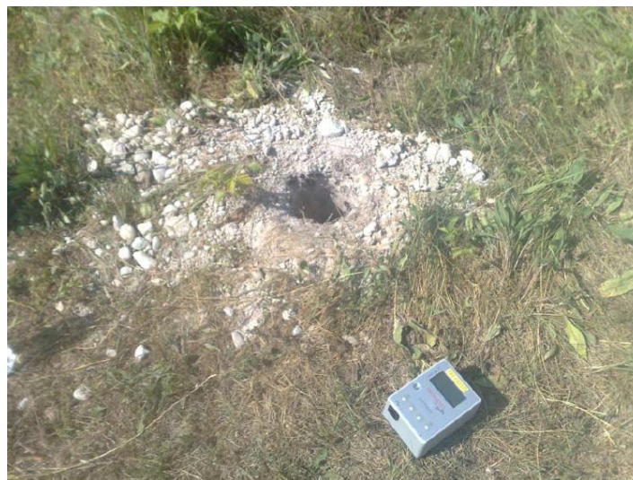
Figure 1. Ambient vibration measurement on the location in Banja Luka (report IZIIS 2009)
