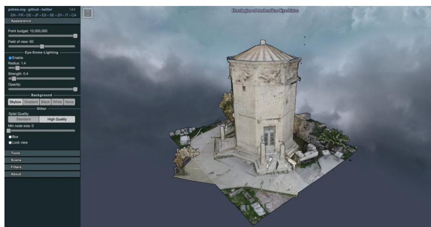
Figure 11. Figure 11. Interactive visualization of the 3D model using the Potree web-based point cloud viewer
