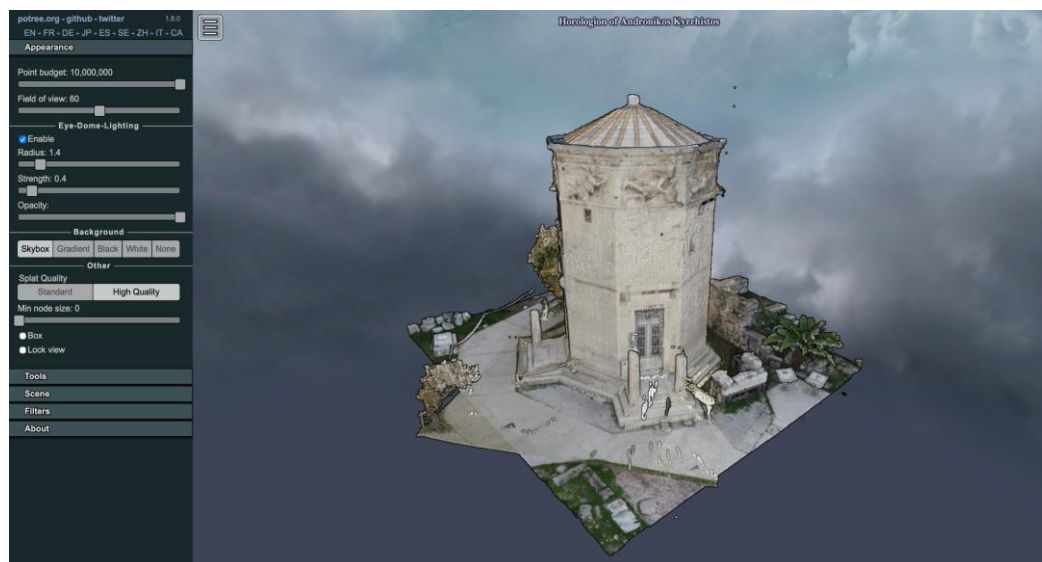
Figure 11. Figure 11. Interactive visualization of the 3D model using the Potree web-based point cloud viewer
