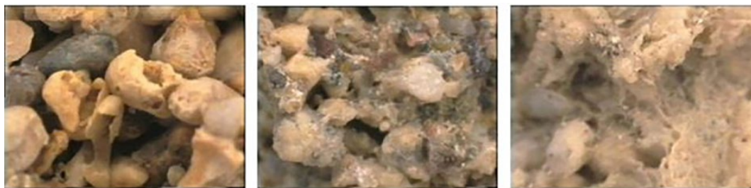
Figure 1. Fiber optic images from consolidation interventions (x50), untreated porous stone (left), treated porous stone with different consolidants (middle and right) [10].
