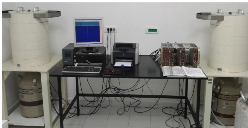
Figure 1. Laboratory for gamma spectrometry in the Centre for Ecotoxicological Research in Podgorica – two ORTEC HPGe spectrometers (photography by author).
