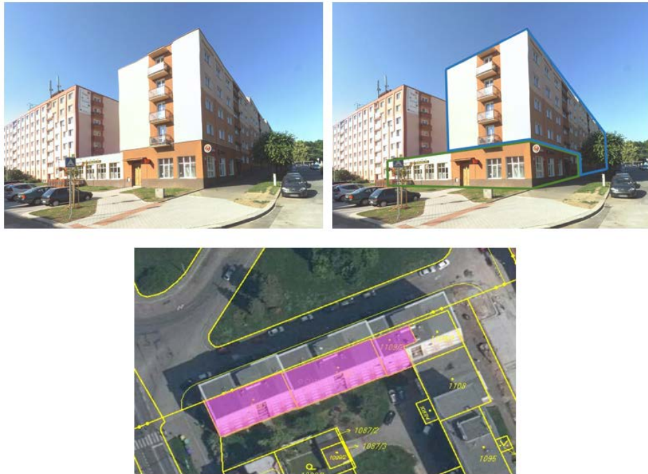
Figure 1. (up left) At first sight one could say that there are two tall buildings and one smaller standing between them. (up right) In fact, there is a building (highlighted in blue), which is partially located above the other building (highlighted in green). (down) The 3D situation depicted on the 2D cadastral map in combination with orthophoto.
