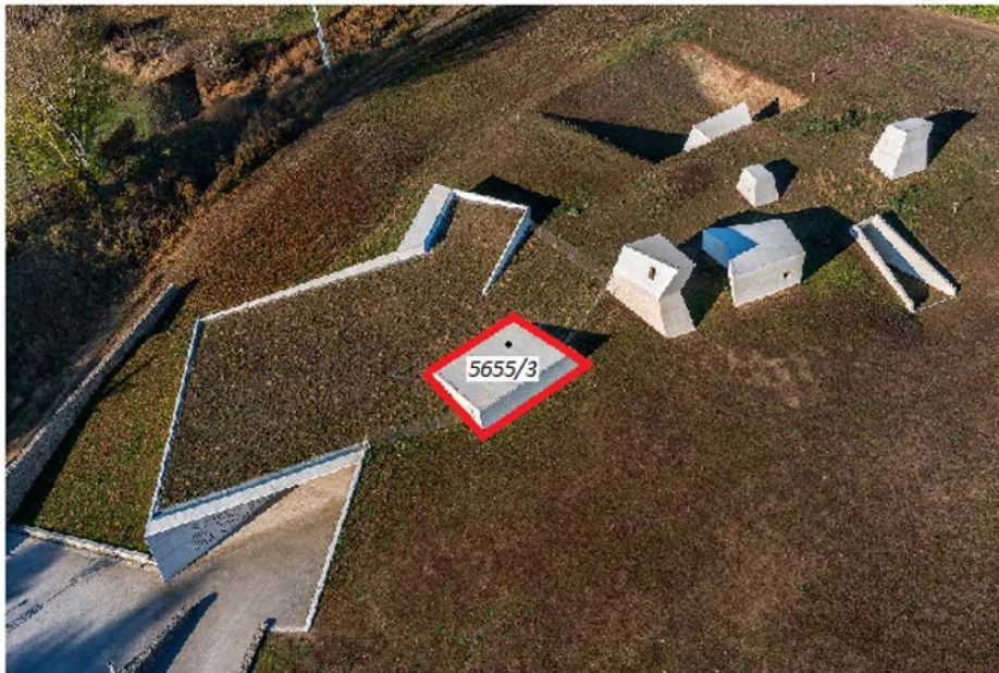
Figure 5. 2D visualization of the boundaries of underground construction (Archeological park Pavlov, Czech Republic) on the cadastral map. Every component of the construction located above ground is displayed on a “separate” building parcel. However, in fact, only one building parcel is registered in the cadastre (here with parcel number 5665/3). (down) The photography of the underground object with components located above the ground. Highlighted in red is the part of the underground object corresponding to the building parcel 5655/3 (source of photography: http://alesjungmann.cz/project/archeopark-pavlov ).
