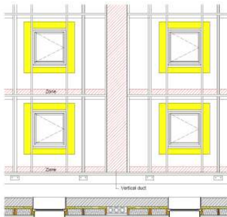
Figure 3 Scheme of prefabricated system for façade retrofitting [7]
