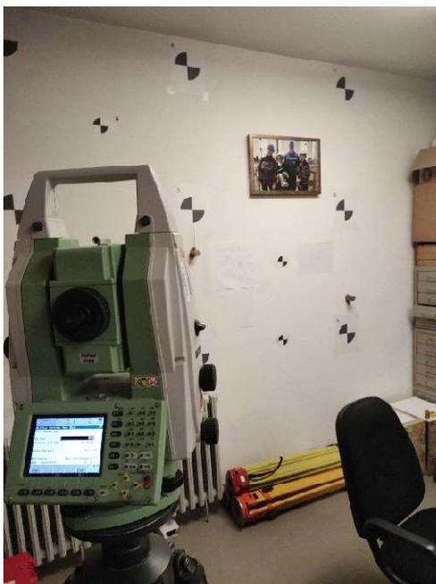
Figure 1. The conditions and total station during measurements
