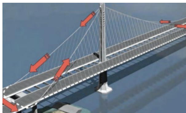
Figure 17. Diagram of load transfer on the Oakland Bay Bridge.
