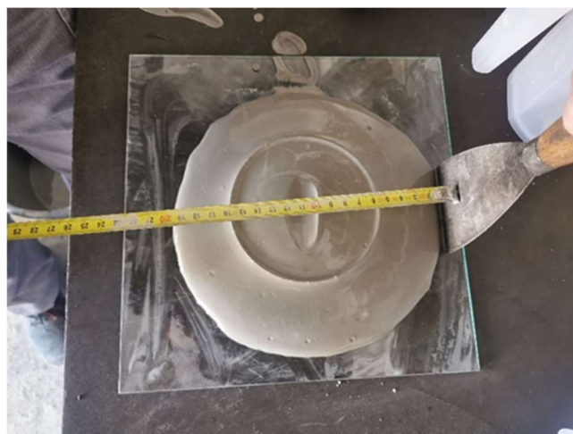
Figure 1. Measurement of the diameter of the mortar spread.
