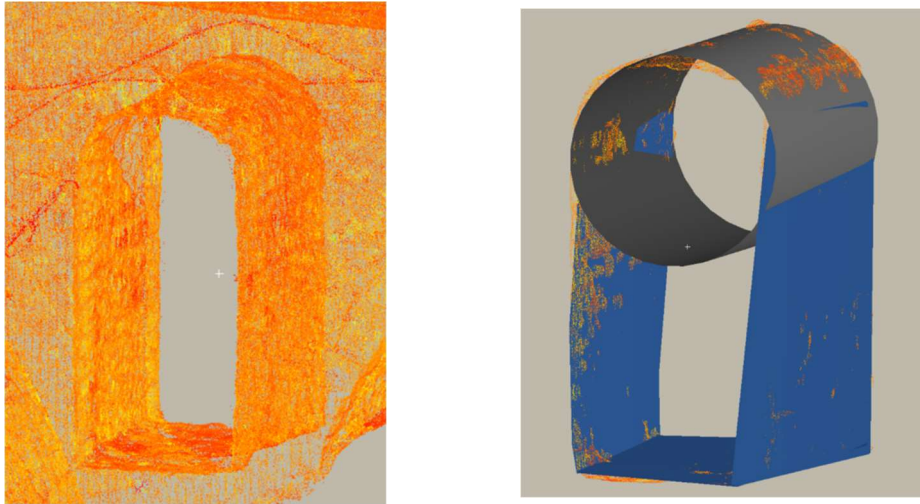
Figure 13. Snapshot of the point cloud of the first relief arch (left) and the modeled surfaces output (right).
