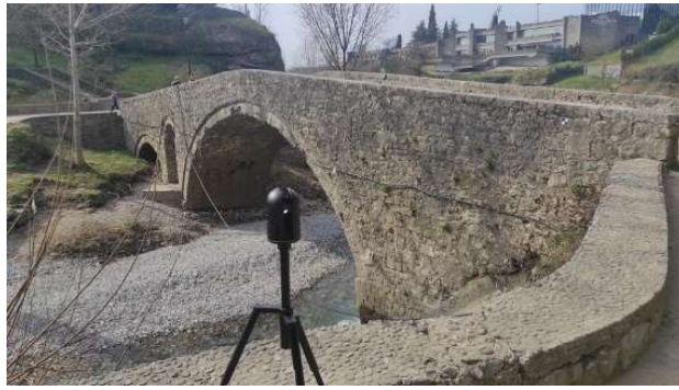
Figure 5. Ribnica bridge during scanning process (authors)
