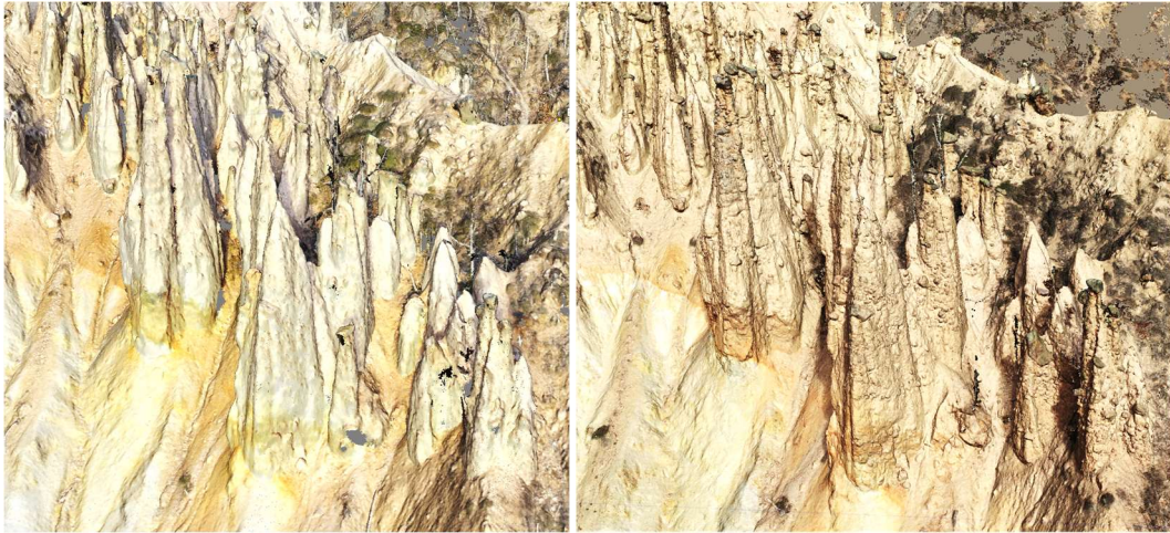
Figure 3. Difference between level of detail between 3D model reconstructed with automated mission flight plan (left) and free flight manual mission flight plan (right)
