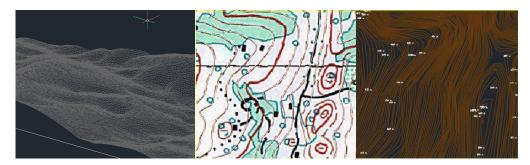
Figure 2. Used datasets (TIN network created from LiDAR data - left, part of a topographic map - middle, contours from open-source data - right)
